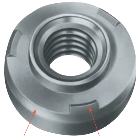
The engineered projections of PEM weld nuts prevent burn-outs in thin sheets
